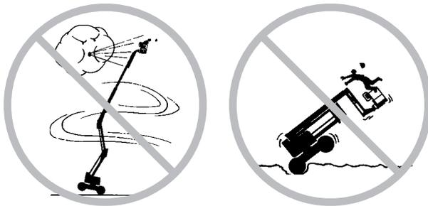
Use extreme care and slow speeds while driving the machine in stowed position across uneven terrain, debris, unstable or slippery surfaces and near holes and drop-offs.
